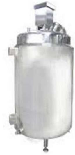
They are used to store various liquid solution at required conditions. In this case they are used to hold oil for frying.
