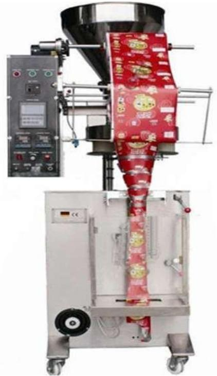
The functioning of machine is simple, it forms an open pouch by two step sealing, followed by filling of chips, nitrogen flushing and final sealing to obtain the namkeen filled packet.
